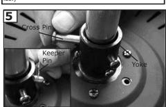
Loosen the 2 set screws in yoke for downrod to slip into yoke. Insert downrod into yoke on top of the Fan Body. Align the hole in the Downrod with the hole in the Yoke. Insert the Pin through the Yoke and Downrod until the point appears on the other side. Install the Keeper Pin
